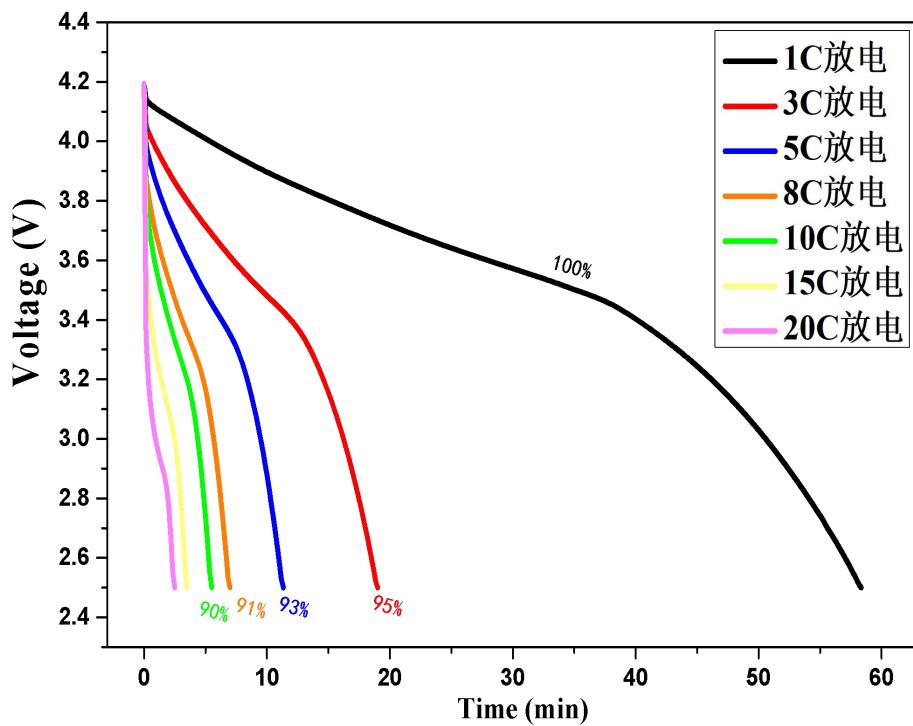
倍率充电性能测试 Charge at different rate
